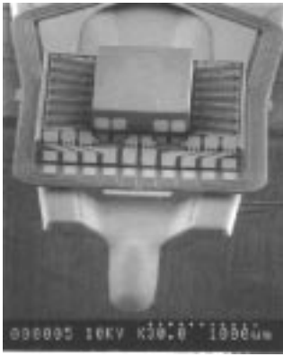
Fig. 1. IBM's electrostatic MA mounted on an integrated lead suspension (Courtesy of L.-S. Fan.).
