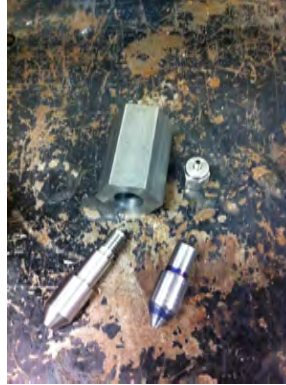
Figure 6: Two machined insert (bottom) and cap (top) used on the engine's fuel rail to open or plug its inlets.
