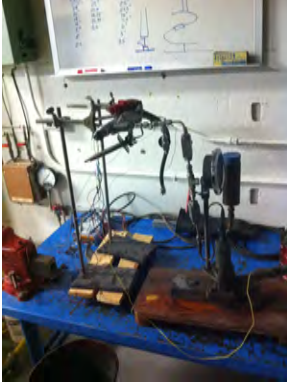
Figure 5: Pressure sensor calibration test setup. Only one of the four fuel inlets of the fuel rail allows flow through to the firing cylinder. See Figure 6 for custom inserts to achieve this flow reduction.
