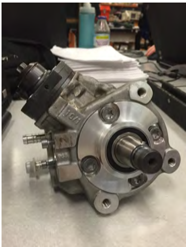
Figure 3: The modified decommissioned Bosch fuel pump.
