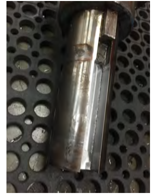
Figure 7: Enlarged keyway on the output shaft of the generator drive line to eliminate the slop of the keystock while spinning.
