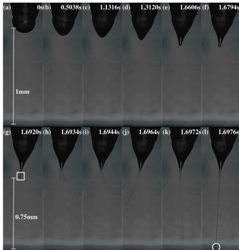
Figure 2. Formation and motion process of charged jet in NFES. Spinneret to collector distance, applied voltage and polymer solution concentration are 1 mm, 1.7 kV and 18%, respectively.
