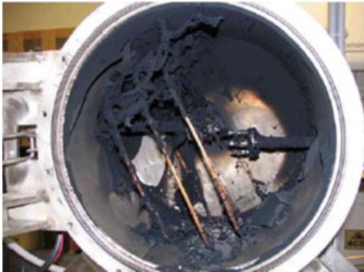
Figure 2. Discharge System Used in the Production of SWCNTs [1]
