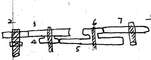
$\frac{\omega_a}{\omega_d} = \frac{\omega_a}{\omega_b} \frac{\omega_b}{\omega_d} = \left(\frac{d_b}{d_a}\right) \left(\frac{d_c}{d_d}\right)$
