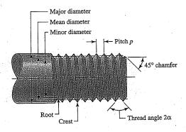
The lead l, not shown, is the distance the nut moves parallel to the screw axis when the nut is given one turn. For a single thread, as in Fig. 8–1, the lead is the same as the pitch.
