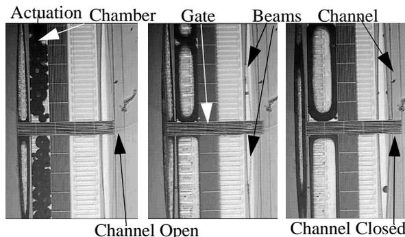
Figure 11. Buckling Beam Valve in both bi-stable positions
