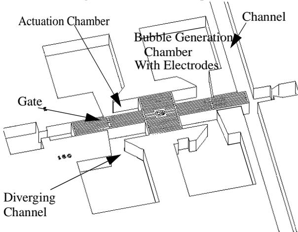
Figure 2. Enlarged Electrode Area Valve Design
