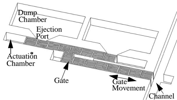
Figure 3. Bubble Ejection Valve Design
