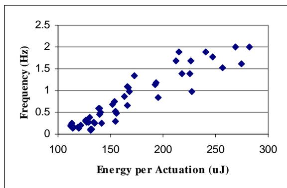
Figure 10. Bubble Ejection Valve Frequency vs. Energy Consumption
