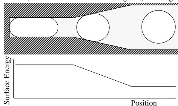
Figure 1. Surface energy of bubbles in confined channels with hydrophilic walls.
