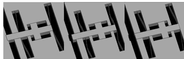
Figure 4. Bi-Stable Buckling Beam Valve Concept
