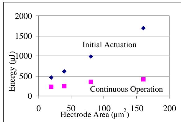
Figure 8. Large Electrode Area Valve Energy vs. Electrode Area.
