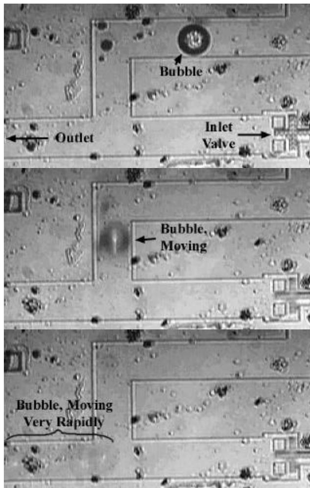
**Figure 6.** (Top) Flow channel with a trapped bubble. (Middle) Motion of the bubble after power has been supplied. (Bottom) Acceleration of the bubble as power is maintained.
