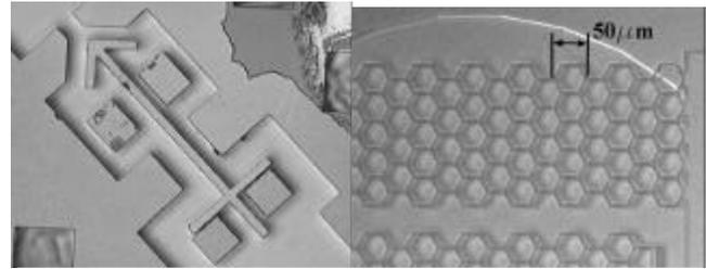
**Figure 3.** (Left) A microfluidic checkvalve. (Right) Fabricated and assembled crack resistant polysilicon heater.
