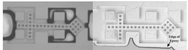
**Figure 4.** (Left) Check Valve after epoxy bonding and before ashing. (Right) Same valve after ashing.
