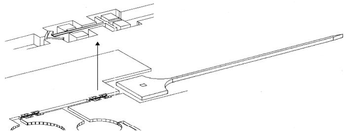
**Figure 1.** Schematic of an integrated micropump/microneedle device. The top shows a closeup of a planar microvalve.
