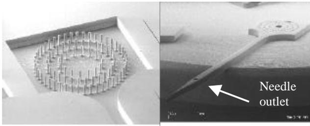
**Figure 2.** (Top) Microneedle fabrication process flow. (Bottom Left) SEM of a microneedle mold. (Bottom Right) SEM of a representative microneedle.
