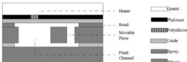
**Figure 5.** Description cross section of the device
