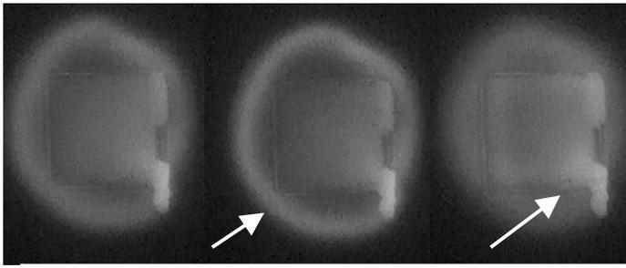
**Figure 7.** (Left) Outlet when no bubble is present in the bubble chamber. (Middle) Change in radius of curvature and collection of fluid at the outlet when the pump is actuated. (Right) Change in the radius of curvature when the bubble collapses. Side view of the fluid bubble is shown below the picture
