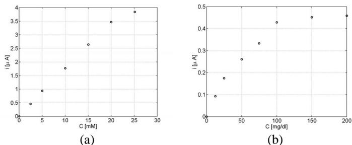
Figure 7. (a) Calibration of the electrochemical sensor with  $H_2O_2$ . (b) Output current versus glucose concentration.
