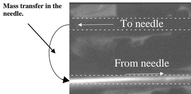
Figure 8. Two microchannels with flow entering and leaving the microdialysis needle after fluorescein dye has equilibrated across the dialysis membrane in the microneedle. The channels are delineated by the dashed white lines. The needle is not seen in the frame but forms a continuous fluid channel to the left of the frame.
