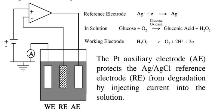
**Figure 1. (Left) Schematic of a three electrode electrochemical sensor. (Right) Summary of reactions which occur in a glucose sensor. Glucose oxidase is bound to the sensor and a current proportional to the glucose concentration is sensed at the Pt working electrode (WE).**
