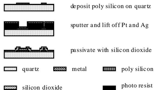
**Figure 6. Simplified process flow for depositing electronics including polysilicon heaters and electrochemical cells onto quartz.**
