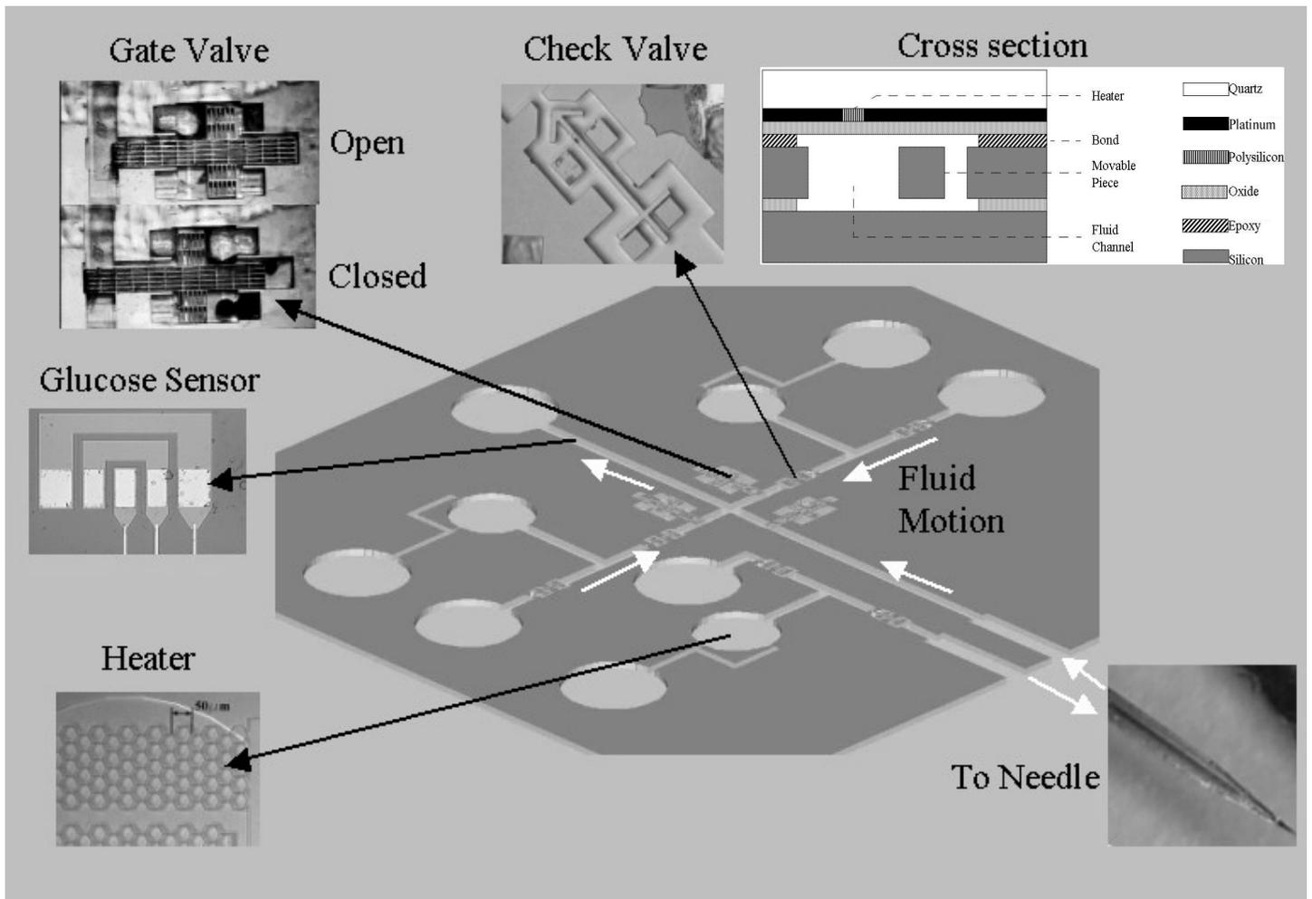
**Figure 4. (Above) Schematic of a three channel sensing chip with integrated components including micropumps, microvalves, glucose sensor and a microdialysis needle. White arrows show the direction of fluid flow in each channel.**
