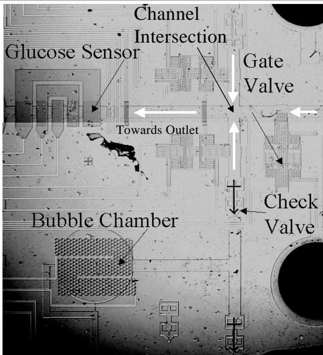
**Figure 5. Composite photograph of the assembled device showing the salient features. The white arrows depict the direction of fluid flow in each of the three channels.**
