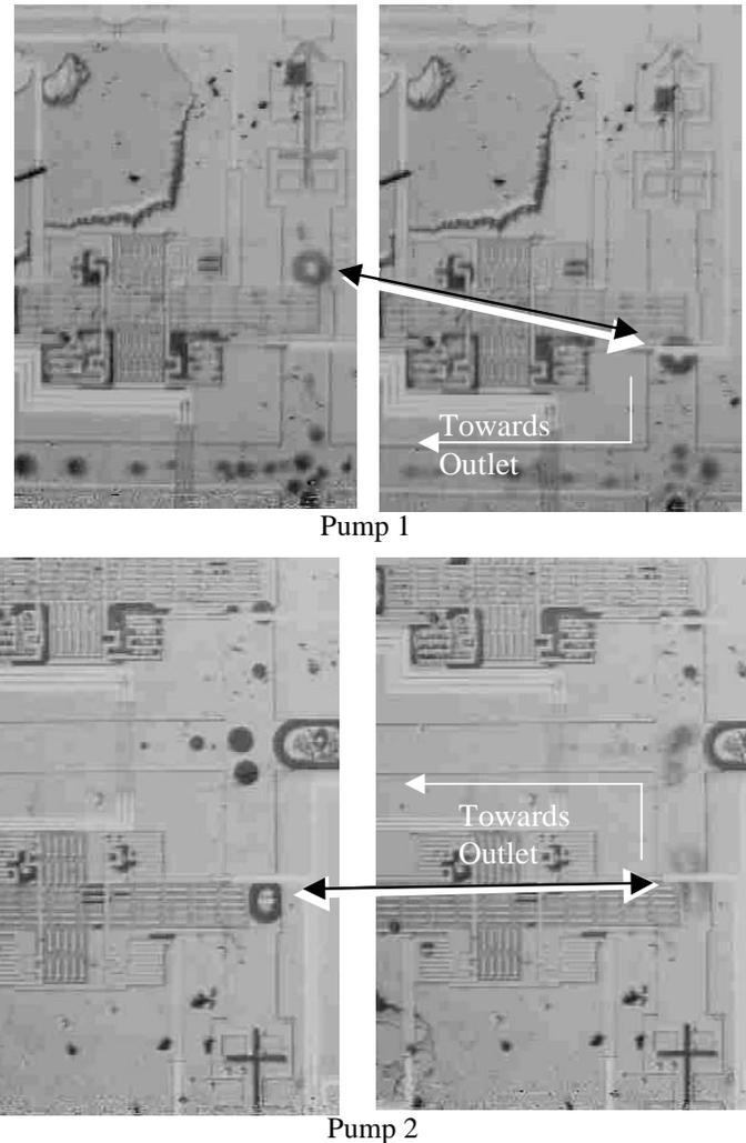
**Figure 9. (Top) A series of frames showing net pumping towards the outlet when Pump 1 is activated. The tracer bubbles can be seen proceeding downwards and towards the outlet. (Bottom) Next Pump 2 is activated. Now the tracer bubbles proceed upwards and to the left towards the outlet.**
