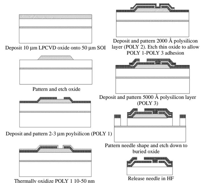
**Figure 3.** Fabrication details of the microdialysis membrane. The microshell is formed over a sacrificial oxide spacer layer. Several polysilicon layers are sandwiched around a thin sacrificial oxide which defines the diffusion channel. Appropriate access holes are etched into the polysilicon layers to allow small MW molecules to permeate across the membrane.
