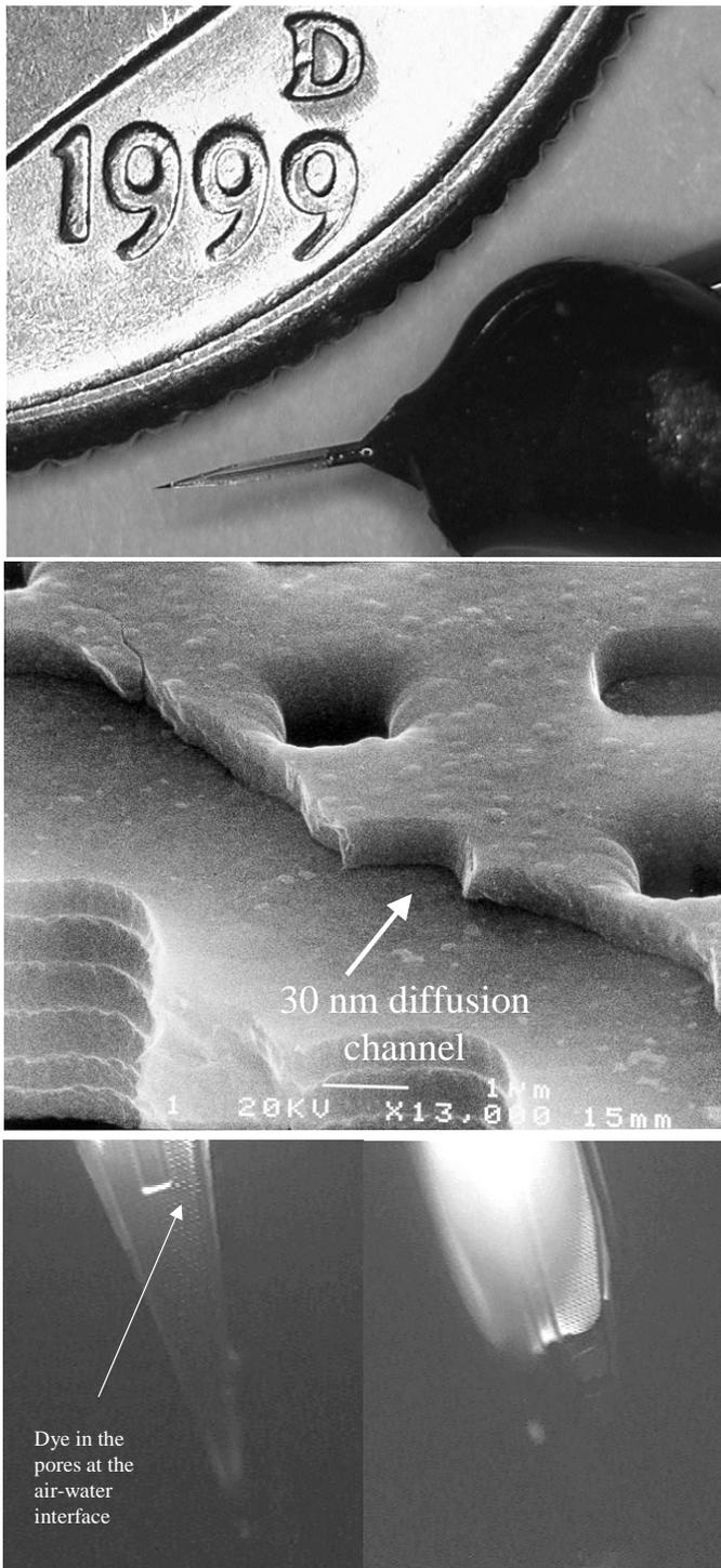
**Figure 2.** (Top) Packaged Microneedle next to a dime for size comparison. (Middle) Diffusion channel membrane. A thin (30 nm) opening can be seen between the polysilicon layers. The layers fractured at different points indicating they are separate. (Bottom) Fluorescent dye emerging from the microdialysis needle. Dye in equilibrium with a water droplet on the needle. Pores can be seen as small dots on the needle surface.
