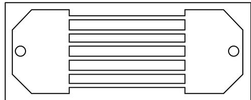
Initial experiments focus on the conformation of the DNA molecule as it is pumped through the device channels. Driven by a syringe pump (Sage Instruments model M362), fluid enters and exits the device via the through-holes; vinyl tubing secured by epoxy connects the pump to the device.
