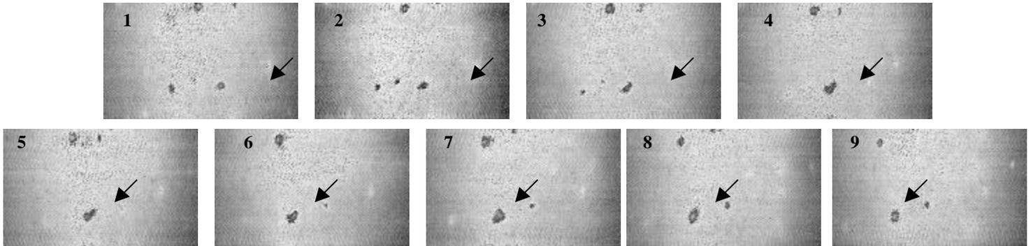
Figure 4: DNA Flow, 3 ml/hr, 0.1 sec/frame
