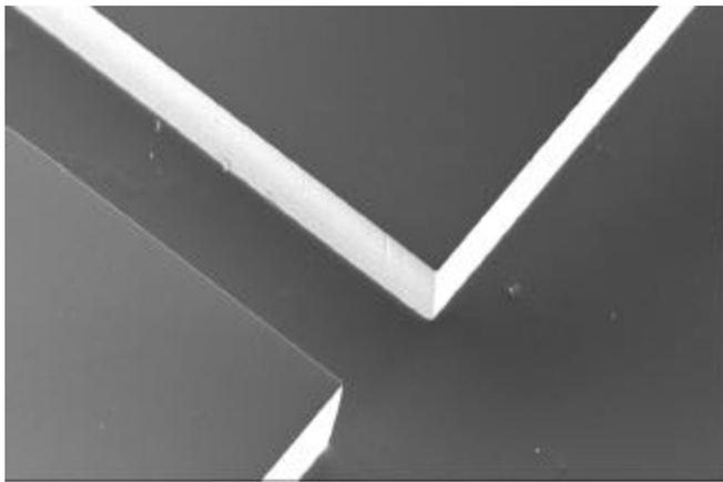
Figure 1a: SEM of device channels, 79X mag.
