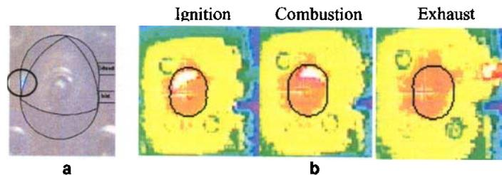
Figure 7. Optical Images of Ignition in MN30 mini-engine
