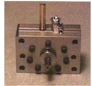
**Figure 10. MN50 Mini-Rotary Engine with Liquid Fuel Carburetor**
