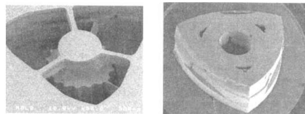
**Figure 11. CWRU Micro-Rotary Engine
