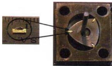
Figure 6. Modified MN30 Rotor with Apex Seals
