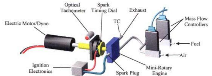
Figure 3. Mini-Rotary Engine Test Bench
