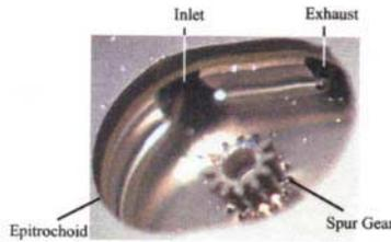
**Figure 12. CWRU Micro-Rotary Engine Housing**
