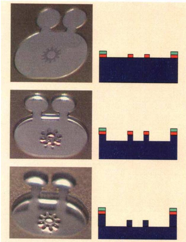
**Figure 3. Micro-rotary engine housing fabrication process.**
