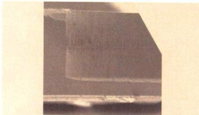
**Figure 7. SEM of cleaved housing wafer. Si DRIE results in 46:1 aspect ratio.**
