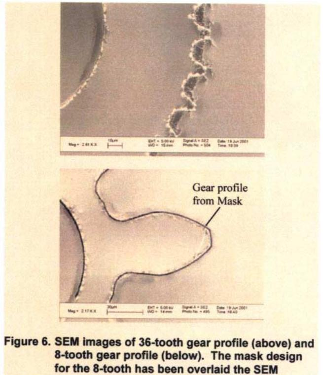
**Figure 6. SEM images of 36-tooth gear profile (above) and 8-tooth gear profile (below). The mask design for the 8-tooth has been overlaid the SEM**
