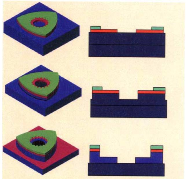
**Figure 4. Micro-rotary engine housing fabrication process.**
