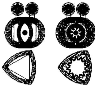
**Figure 2. Micro-rotary engine housing-rotor mask designs**
