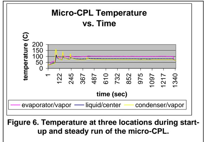
**Figure 6. Temperature at three locations during start-up and steady run of the micro-CPL.**
