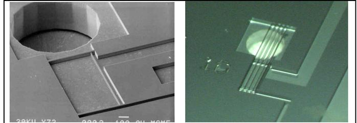
**Figure 2. The evaporator section of the first generation micro-CPL without a cover (left) and with the cover showing the wicking structure (right).**
