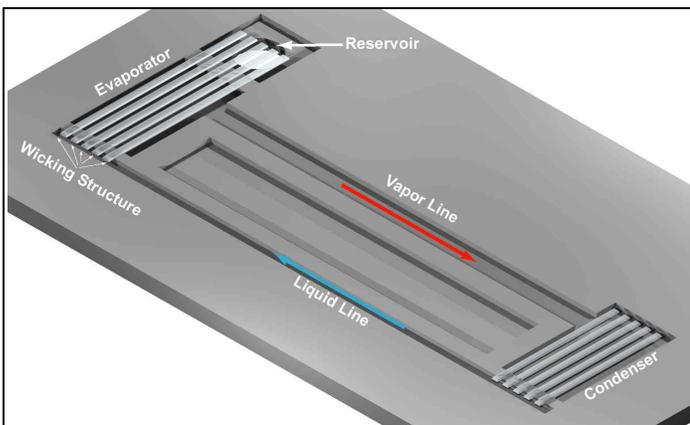
**Figure 1. Schematic of the micro-CPL. The fluidic channels (gray) are fabricated from silicon, while the wicking structure (white) is etched into a borofloat glass cover plate**
