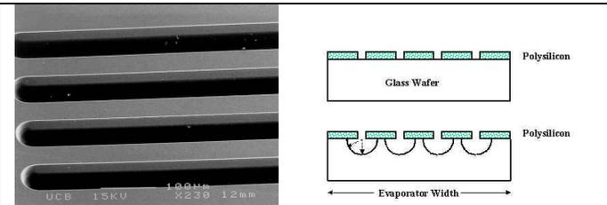
**Figure 4. Wicking structure in the glass cover plate (left) and fabrication approach (right) that determines the geometry of the wick structure.**
