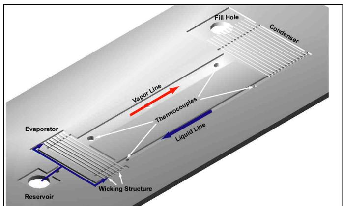
**Figure 3. Schematic of the second generation micro-CPL.**
