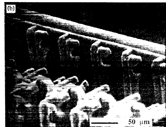
Fig. 5. (a) A SEM photograph of 3-D fabrication on Teflon ® FEP: cantilever array within microfluidic devices. (b) A SEM photograph of 3-D microstructure etching with an incident beam of 45^\circ within microfluidic devices.
