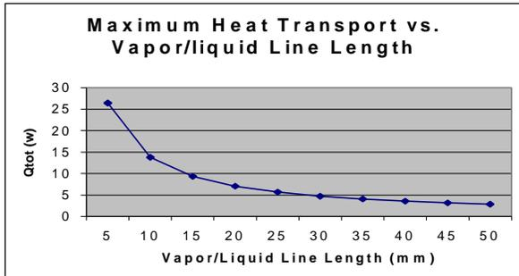
**Figure 2.** Maximum transport distance for 150x150 micron liquid and 450 x 150 micron vapor lines.
