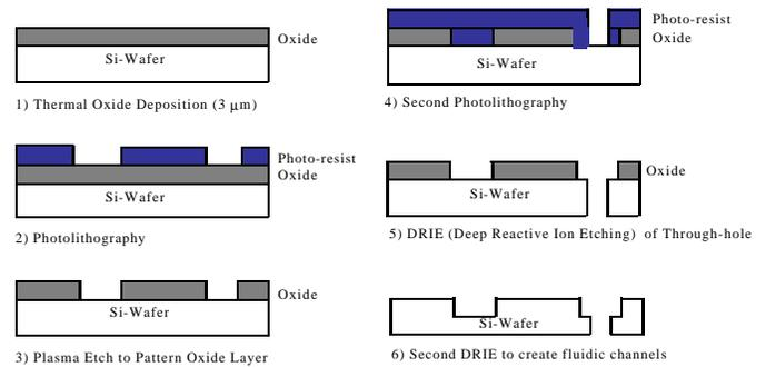
**Figure 4.** Fabrication process for the silicon wafer
