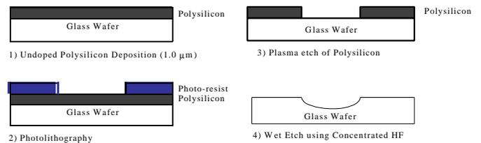
**Figure 5.** Fabrication process for the glass wafer
