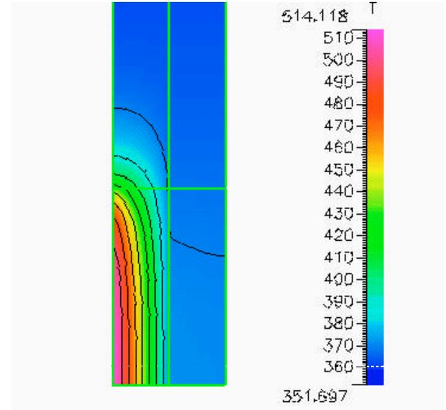
**Figure 10.** Temperature profile of a cross-section of the blank glass (left) and silicon (right) wafers. The bottom is the center of the wafer (where the heat source is placed on the glass side). Due to scaling, the outer sections of the wafers are not shown.
