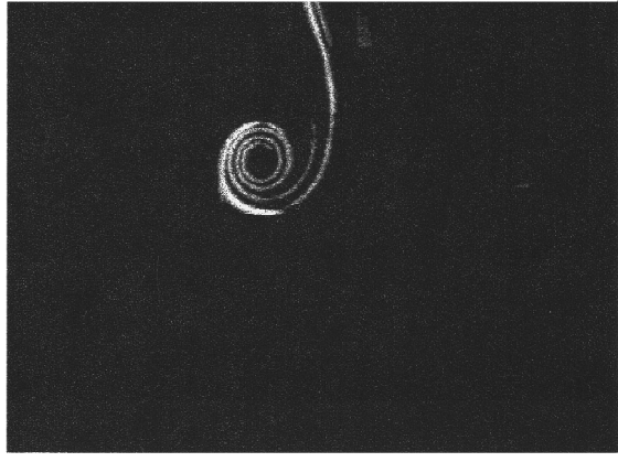
FIG. 2. Dye entrained into a vortex ring (Reynold's number of 4000).
