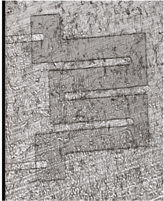
Fig. 32.17 Piezoresistive strain sensor on steel substrate
