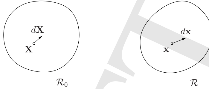
Figure 3.7: Mapping of an infinitesimal material line elements d\mathbf{X} from the reference to the current configuration.
